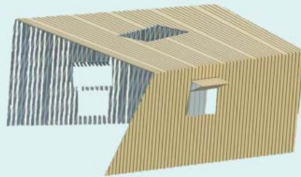
WOODEN SKIN - SUPPORTED BY MOMENT CONNECTED BEAMS
