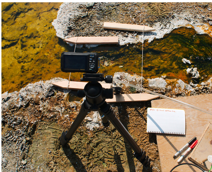
Figure 3.5: A photo of the experimental set-up used to measure stream velocities. Video was taken of the a buoyant object transiting the demarcated area. A frame-rate analysis allowed stream velocity to be calculated. In this photograph, flow is from left to right.
