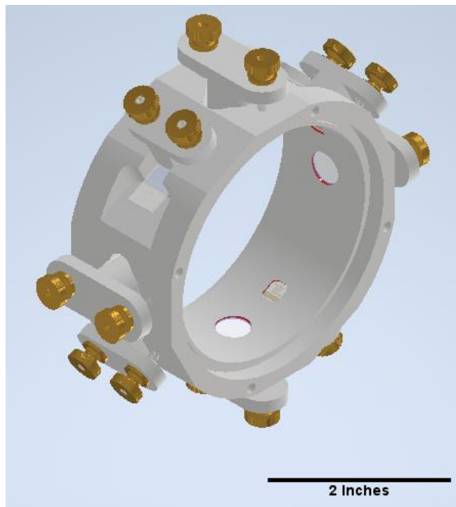
Figure 12: 3-inch tangential AGBR coupon ring with coupons and sensors mounted.
