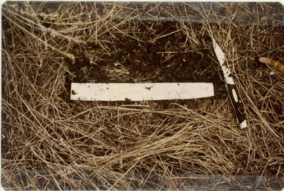
Figure 16. 'Tempilstik' packet being placed below the soil surface.
