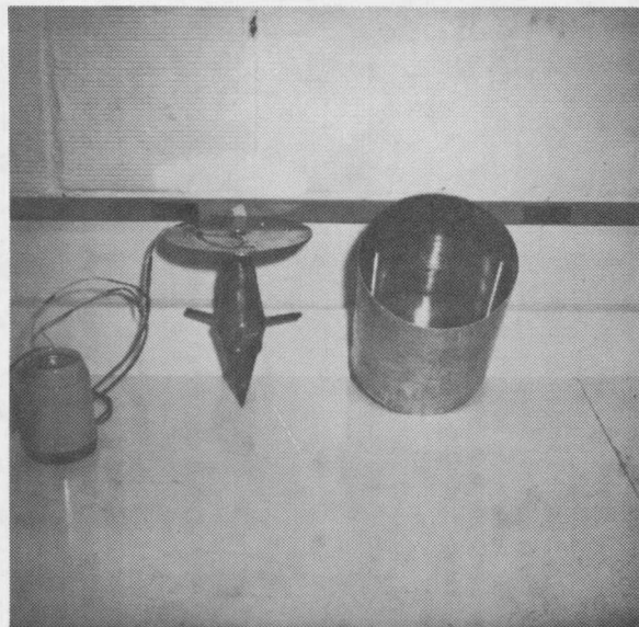
Figure 3.5 Upper--Diagram of blackbody calibration chamber. Lower--Photograph of the blackbody cavity and its housing.
