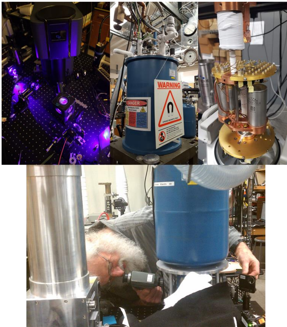
Figure 3.2. Five different cryostats used in this work. Top Left: Montana Instrument's C2 closed cycle Gifford-McMahon system. Top Center: Oxford SpectrumMag helium bath cryostat. Top Right: PhotonSpot's helium sorption fridge. Bottom: Cryomech's closed cycle pulse tube in the silver cylinder and Roger Macfarlane aligning a beam through an Oxford Optistat.
