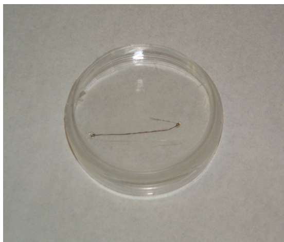
Figure 67. K-PtOx pulled from a capillary tube and secured to a plastic Petri dish with solder.
