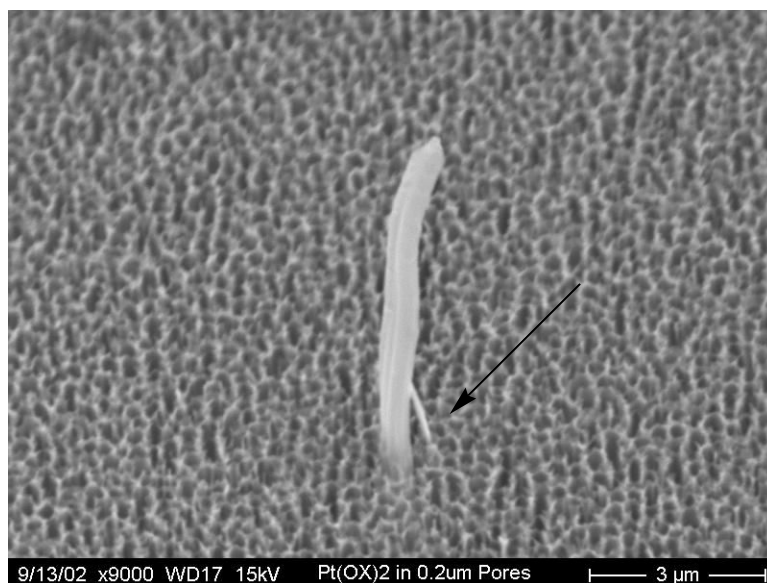
Figure 102. SEM image of a collection of K-PtOx polymers forming a larger polymer (x9000 Mag.)
