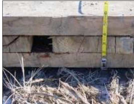
Figure 3. Cross section of an oak mat constructed from individual oak boards.
