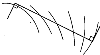
Figure 11. Magnified view of one step in the conjugate gradient technique: a step starts off in the local gradient direction, perpendicular to the contour lines, and traverses a straight line until a local minimum is reached, where the line is parallel to the local contour lines.
