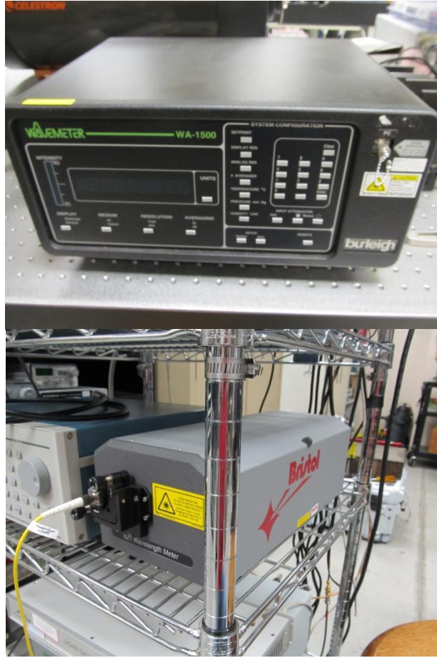
Figure 22: Burleigh WA-1500 (Left) and Bristol 621 (Right) wavemeters used for online laser locking. The Bristol 621 replaced the WA-1500 for the Kevin Dome measurements described in chapter 4.
