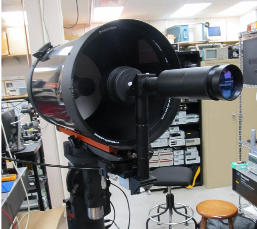
Figure 28: Another photo of the beam expander mounted to the telescope. The beam is entirely contained within SM1 optical tubing until it has been expanded to an eye-safe diameter of 5 cm.
