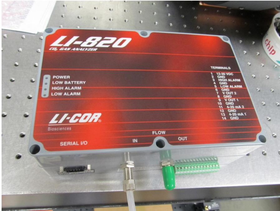
Figure 41: LI-820 gas analyzer made by LICOR used for carbon dioxide measurements to compare to the DIAL.
