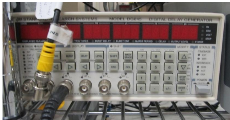
Figure 21: Pulse train generator used for setting the pulse repetition rate and pulse duration control signal for the AOM.
