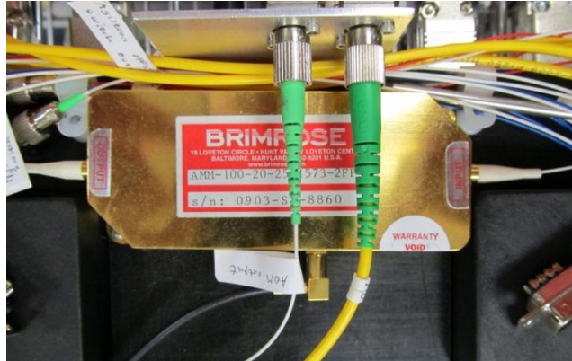
Figure 20: Brimrose AOM used to generate the seeding pulse train for the EDFA.
