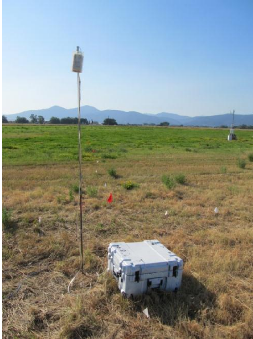
FIGURE 62: Picture of the LI-820 in the field. The LI-820 was run off of a battery in a weatherproof box. Air was pumped through the LI-820 with a small electric air pump elevated off of the ground.
