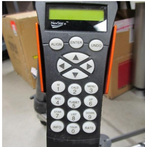
Figure 39: Hand controller that interfaces the Labview control with the motorized telescope base for PC controlled scanning of the DIAL's pointing direction.
