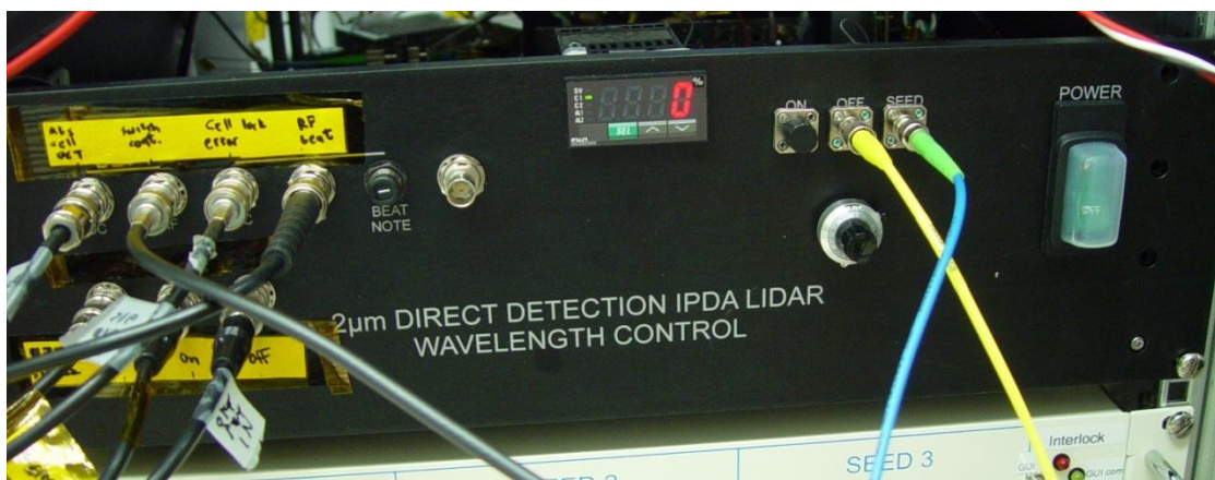
Figure 83: Photo of the wavelength control box
