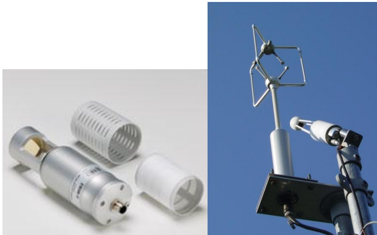
Figure 6: Left: Open path infrared CO 2 analyzer 36 Right: Eddy covariance analyzer 37 Eddy covariance instruments measure not only the concentration of gas, but, estimate the flux of the gas of interest by correlation between measured wind currents and concentrations. These instruments are useful for sequestration sites since they do not make physical contact with the surface whose gas flux is being measured, are autonomous, and are more sensitive to scales of m 2 to km 2 . 38
