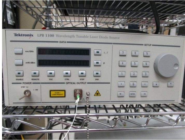
Figure 23: Tektronics source used to maintain EDFA operation with pulsed seed laser signal.
