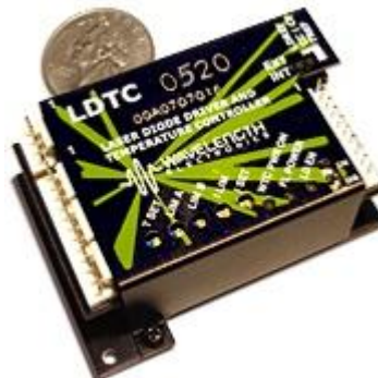
FIGURE 102: The proposed Wavelength Electronics combination laser diode and TEC controller replacement for the ILX laser diode drivers.
