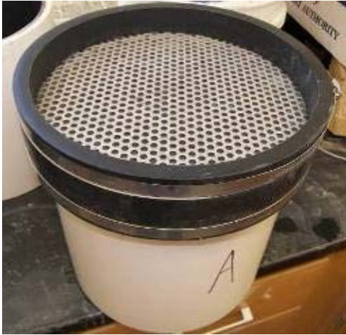
Figure 24. Support plate for bottom of specimen mold.
