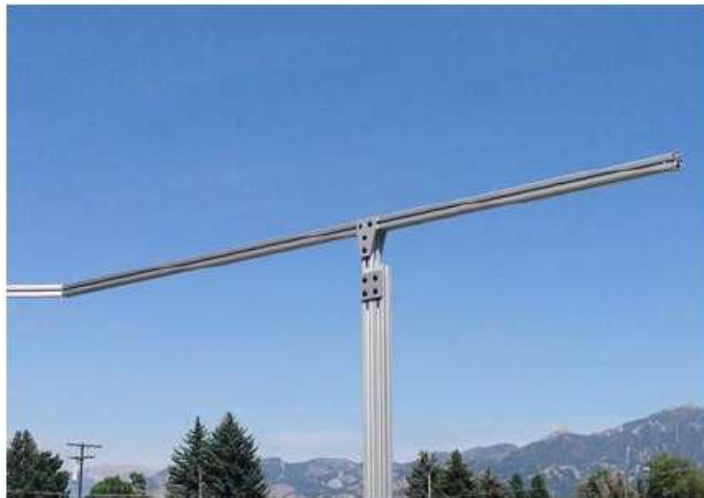
Figure 3.1.2: 3 meter elevated aluminum frame with expandable arms
