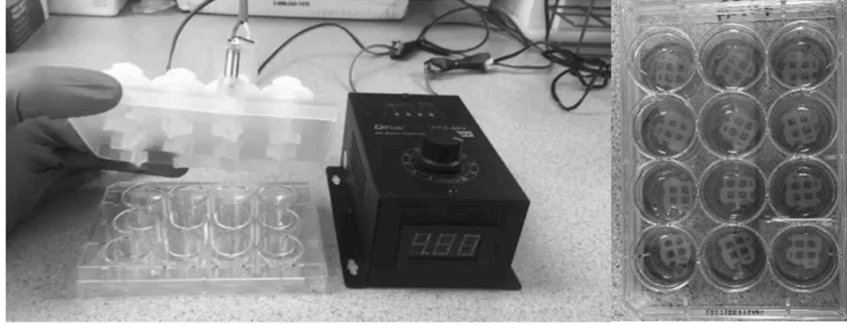
Fig. 2. Spinning bioreactor and speed controller (left), and scaffolds in a 12 well plate (right).
