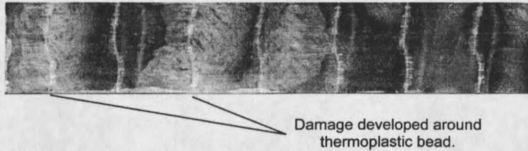
Figure 30. Damage developing around thermoplastic beads as a result of fatigue loading, R=0.1 .
