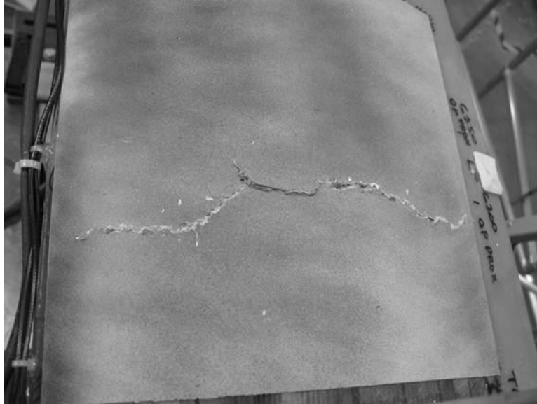
Figure 51: Fatigue failure of BRC blade near an OP wave placed in the spar cap (see Riddle, 2013 for more detail).
