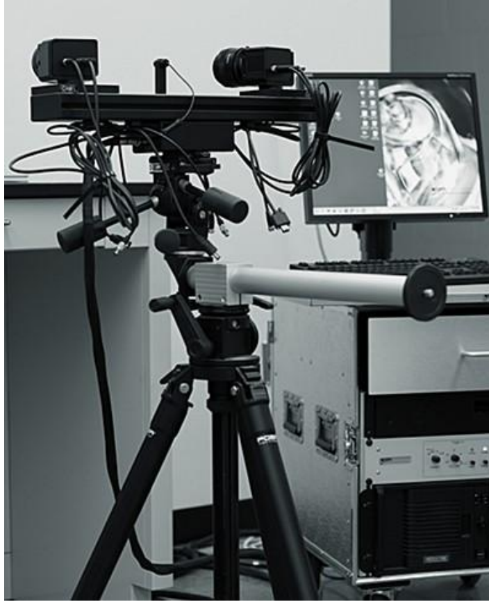
Figure 30: Aramis digital image correlation (DIC) system utilized during entire BMT effort (Aramis, v6.2).
