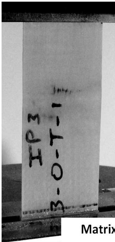
Figure 37: Damage progression of IP Wave 1 with initial damage accumulating at the areas where fibers are not continuous through the length of the sample.
