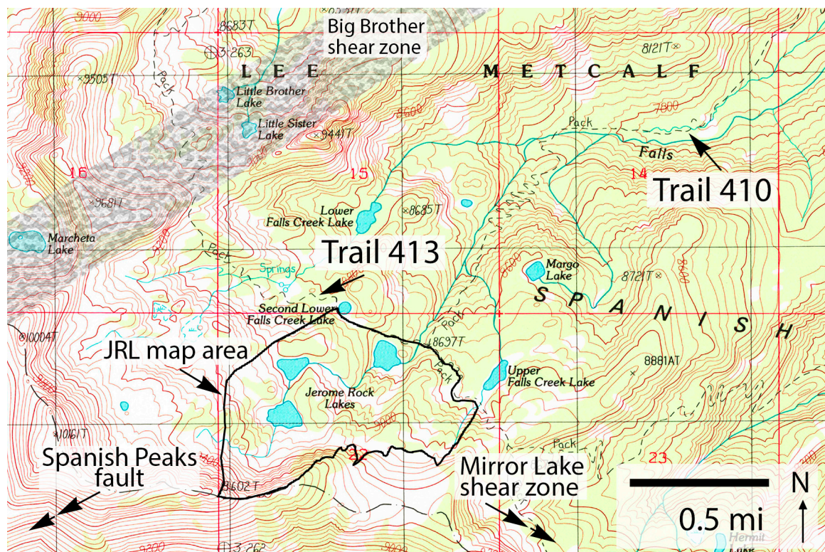
Figure 1: Detail of the Willow Swamp 1:24,000 USGS topo map. The extent of the bedrock map developed by this study is outlined in black. The approximate trace of the Big Brother shear zone is shaded in grey. Directions towards the nearby southeast-striking Spanish Peaks fault and the northwest-striking Mirror Lake shear zone are indicated by the double arrow. Trails no. 410 and High Lakes trail no. 413 are indicated.
