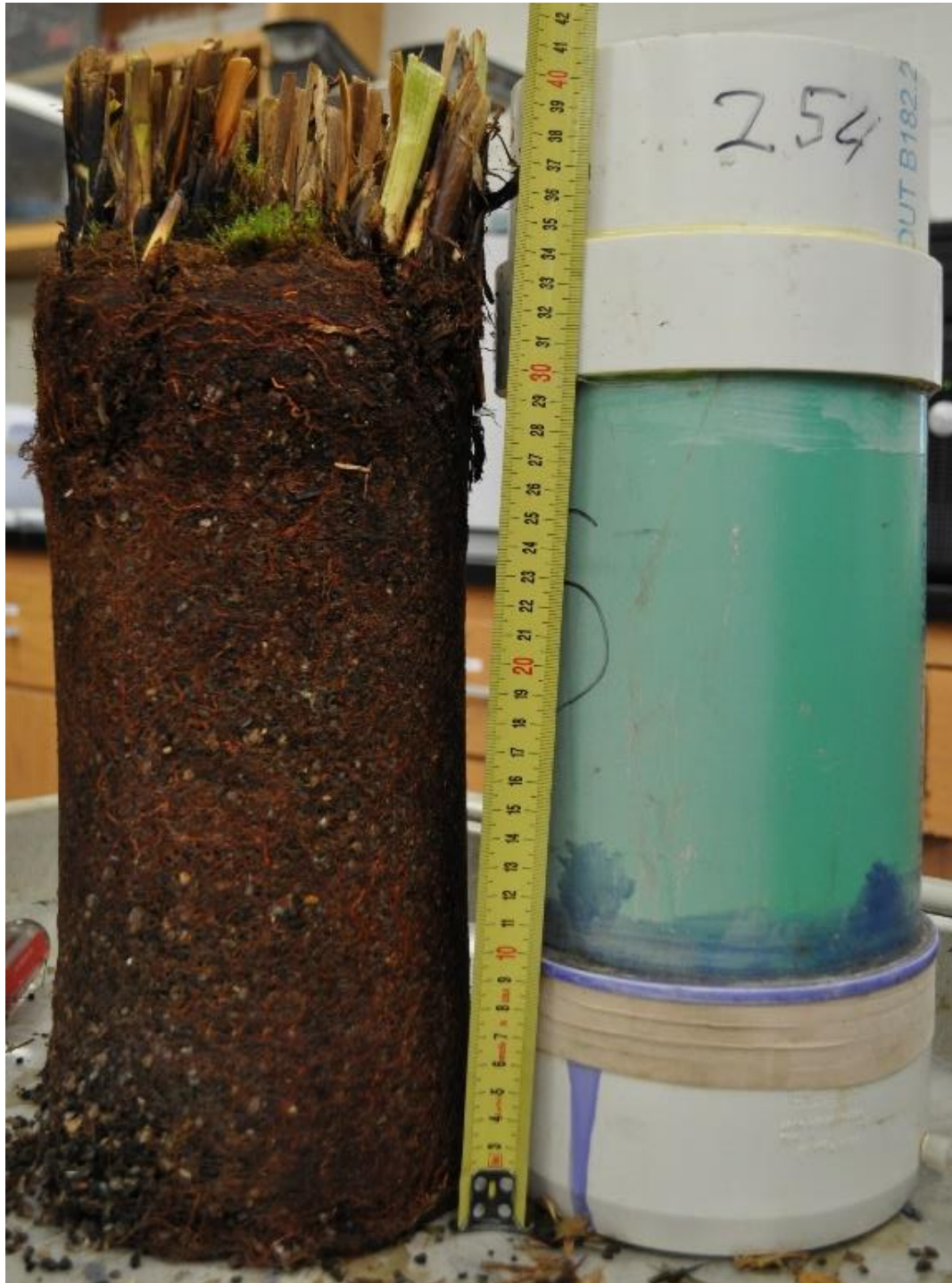
Figure 12. Schoenoplectus OC2x treatment removed from column during destructive sampling. The root bound nature of the subsurface can be seen by both the mat of roots against the column wall, and the ability of the roots to self-support the gravel.
