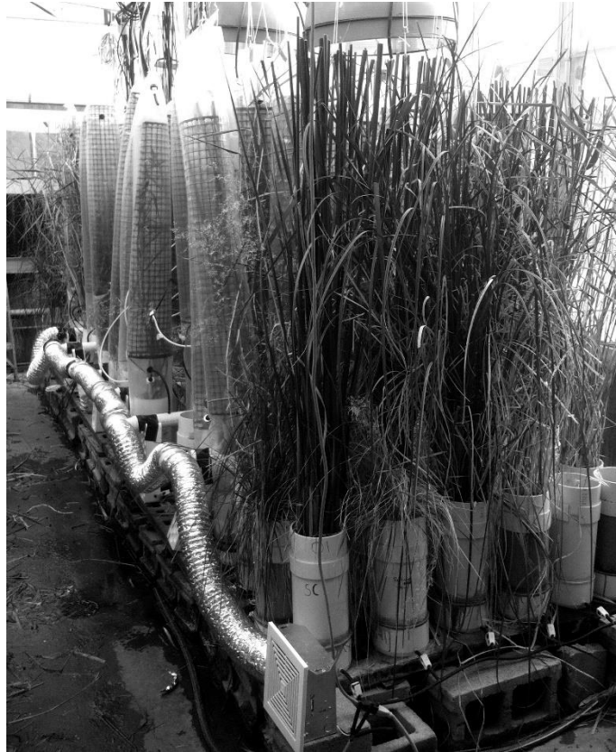
Figure 1. Experimental set-up with low pressure blower system and headspace sample bags in place. Photo from the 24 °C sample period in 2013.
