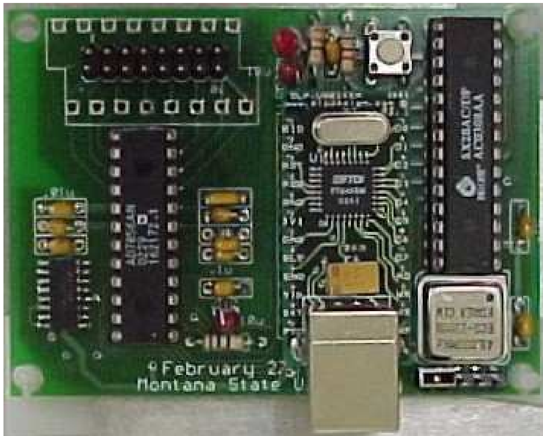
Figure 5: The sampling board converts the data into the digital domain and transmits that data to the computer.
