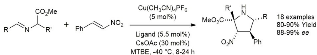
Figure 1.9 Umpolung synthesis of enantioselective pyrrolidines via 1,3-dipolar cycloaddition. 57
