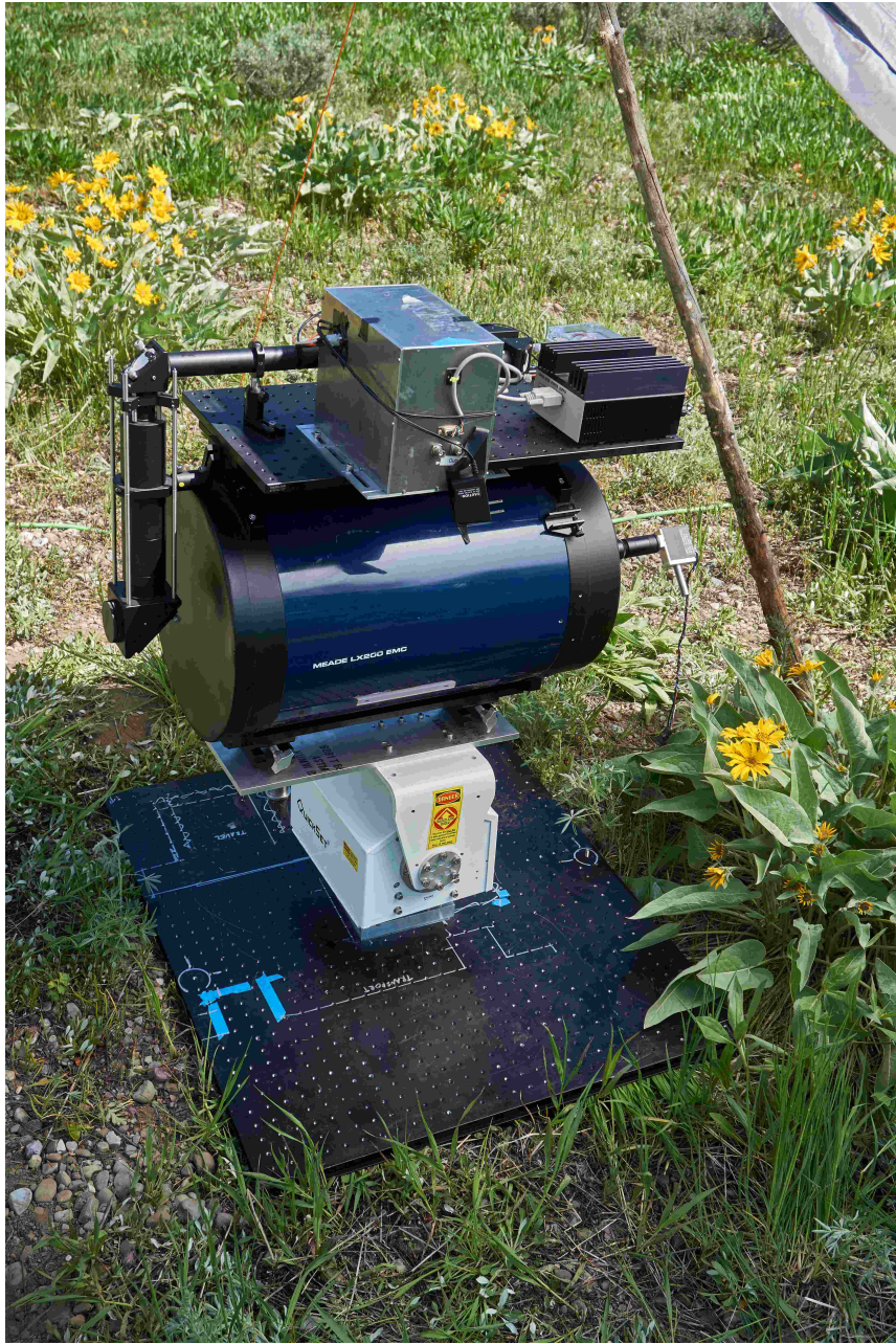
Figure 2.1: The lidar system setup shows the transmitter and receiver sitting atop a scanning mount. Photo courtesy of Kurt Fristrup
