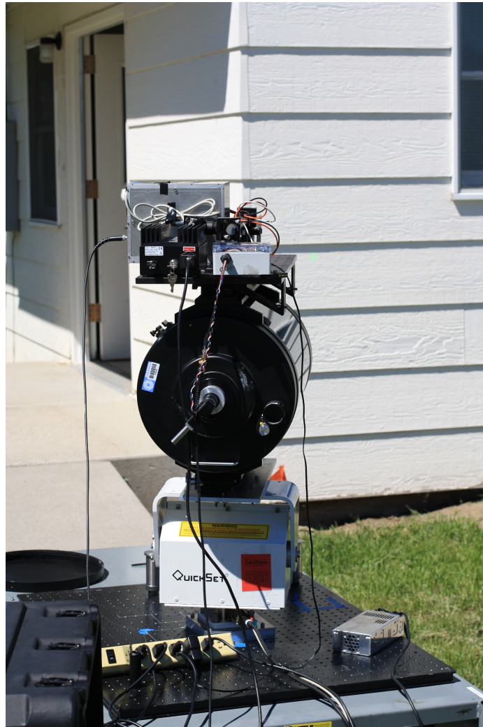
Figure 4.13: Photograph of instrument prior to departure to AMK Ranch. The transmitting optics sat atop the receiving telescope and all of that was attached to a scanning mount.
