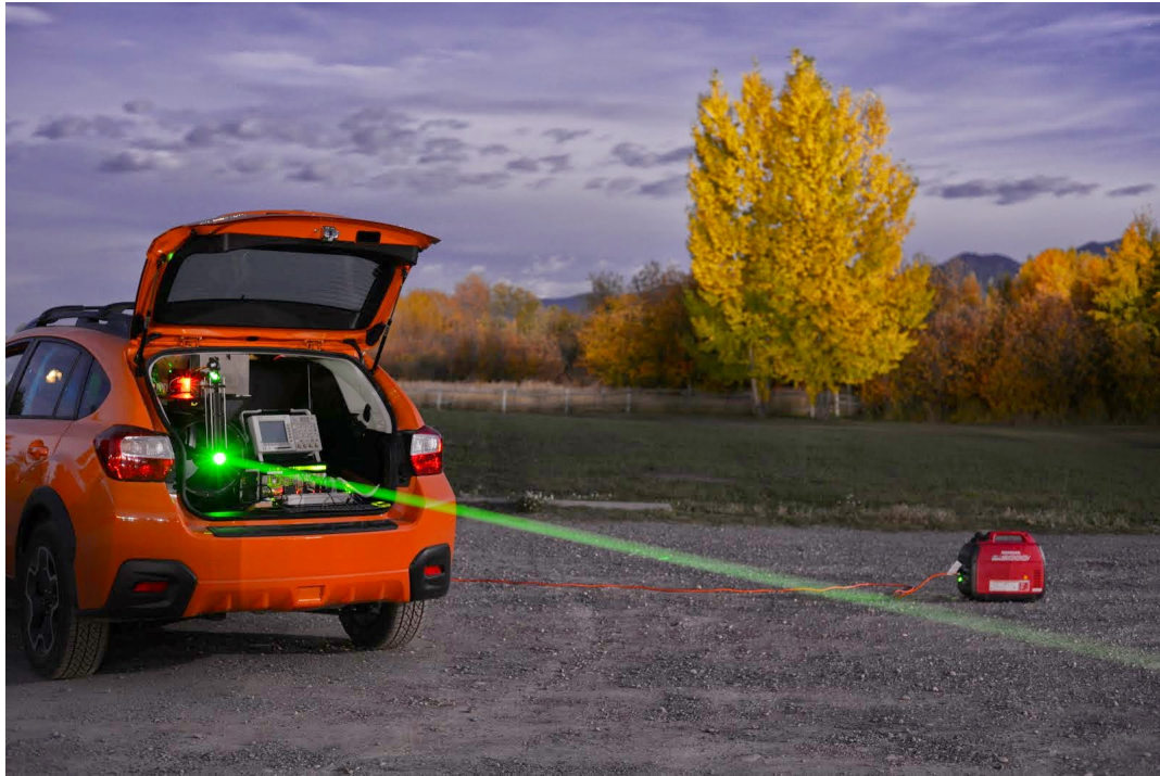
Figure 4.8: Photograph of instrument inside of car with power coming from an external generator. Photo courtesy of Joseph Shaw
