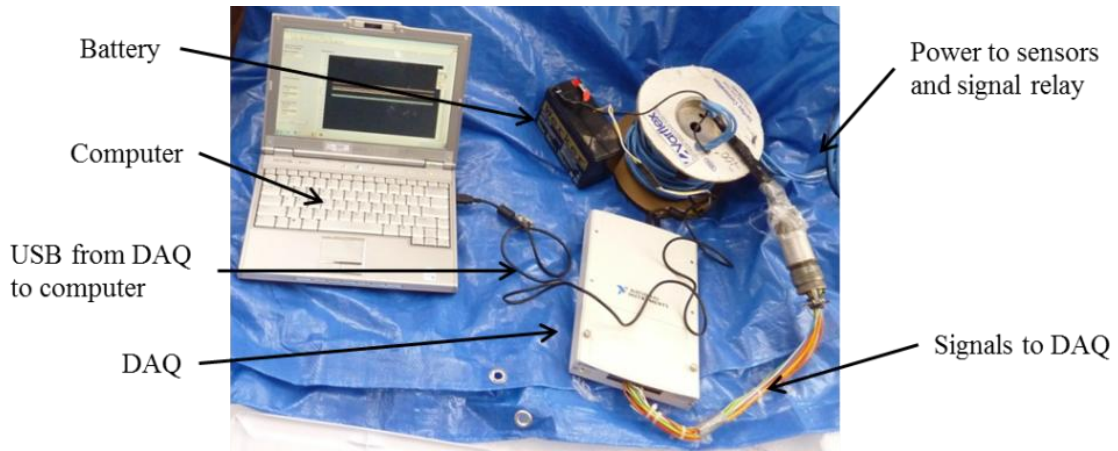
Figure 8 Data acquisition setup for testing season 2010-2011 soft slab snow investigation.
