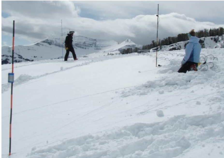
Figure 4 One of the testing sites at Big Sky resort for hard slab snow conditions conducted 2011-2012. The charge is elevated 1 m (left foreground) and the sensor placement as shown was the season testing standard.
