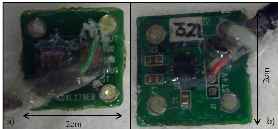
Figure 7 Accelerometers utilized for the 2011-2012 testing season. a) dual axis ADXL 278 accelerometer and b) a dual axis ADXL 321 accelerometer.
