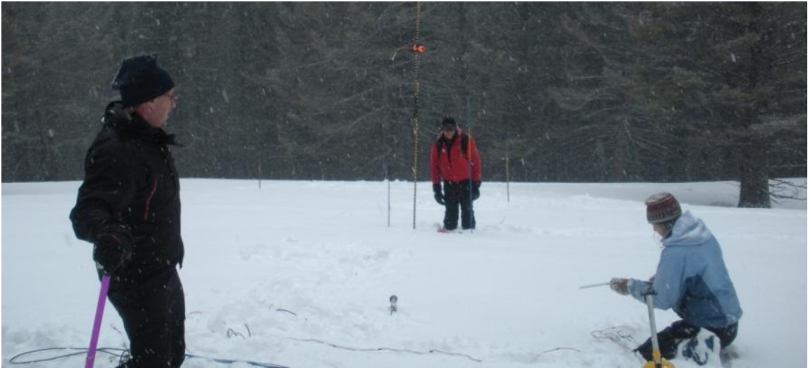
Figure 3 Photo taken during sensor placement at Bridger Bowl during the 2010-2011 testing seasons. This site was selected for soft slab testing. The explosive for this test was elevated 2 m above the surface. While research personnel handled instrumentation, snow safety personnel conducted all explosive handling tasks.
