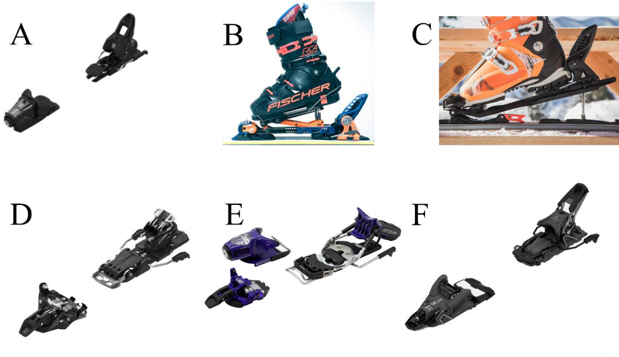
Figure 1. Examples of common binding options for ski mountaineering. A) Alpine binding with DIN settings, must be used with binding B for uphill travel, B) Adapter binding being used in an alpine binding for uphill travel, C) Frame touring binding, entire binding attaches to toe and heel for uphill and downhill travel, D) Pin binding, E) CAST binding with interchangeable toe piece (pin toe piece for uphill, frame toe piece for downhill), F) Freeride hybrid binding, toe piece mechanism moves to expose ‘pins’ for uphill travel, and closes to enclose the toe in a frame style for downhill travel with DIN settings.
