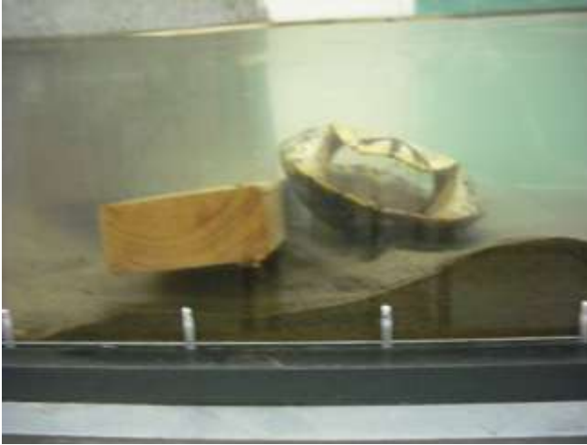
Figure 4.5. The “log jam trial”. A piece of wood (5 cm x 10 cm) is used to model a log jam in the channel. The shell would have continued rolling over onto the plastron if not obstructed. Flow direction is towards the left.
