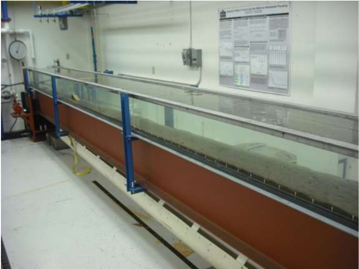
Figure 4.3. The flume in the Engineering Department at Montana State University which was used for observing the transport of extant turtle shells.
