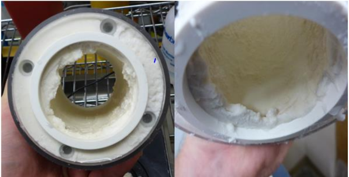
Figure D-2: Post experimental deconstruction of the Wellbore Analog Reactor used for Analog Experiment 1. A large amount of precipitation was found in and around the perforations at the bottom of the reactor.
