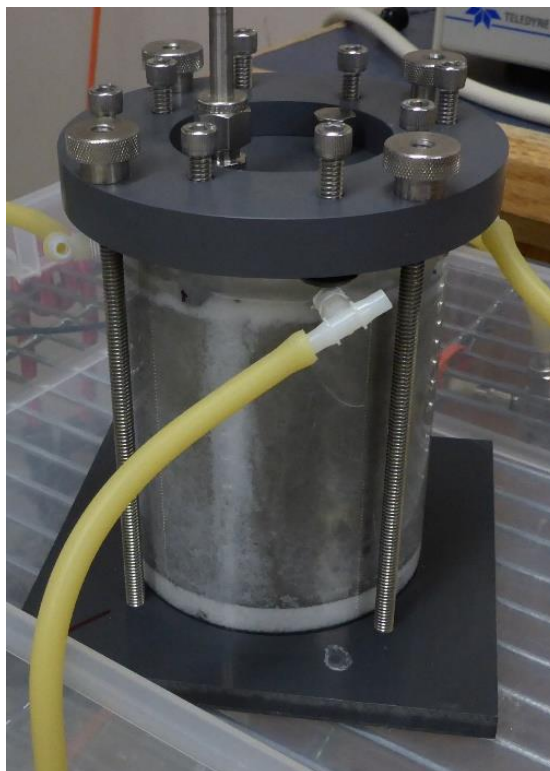
Figure D-1: Instantaneous precipitation, seen as a white flock, occurring during the first injection of calcium containing media.
