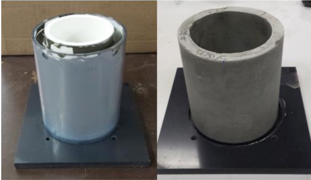
Figure 4: Cement casing in the wellbore mold during (left) and after (right) curing.
