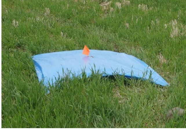
Figure 4.2. Tarp placed in field to locate data points on hyperspectral data. Blue tarps also provided reference for atmospheric correction.
