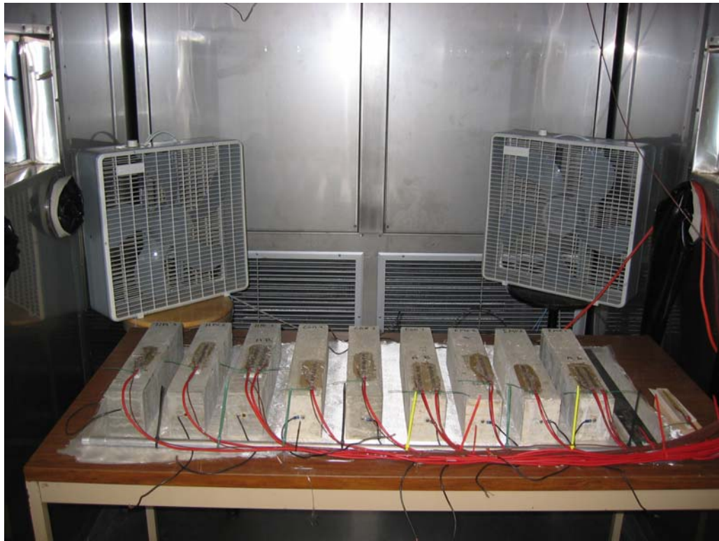
Figure 8. Specimens placed in environmental chamber.
