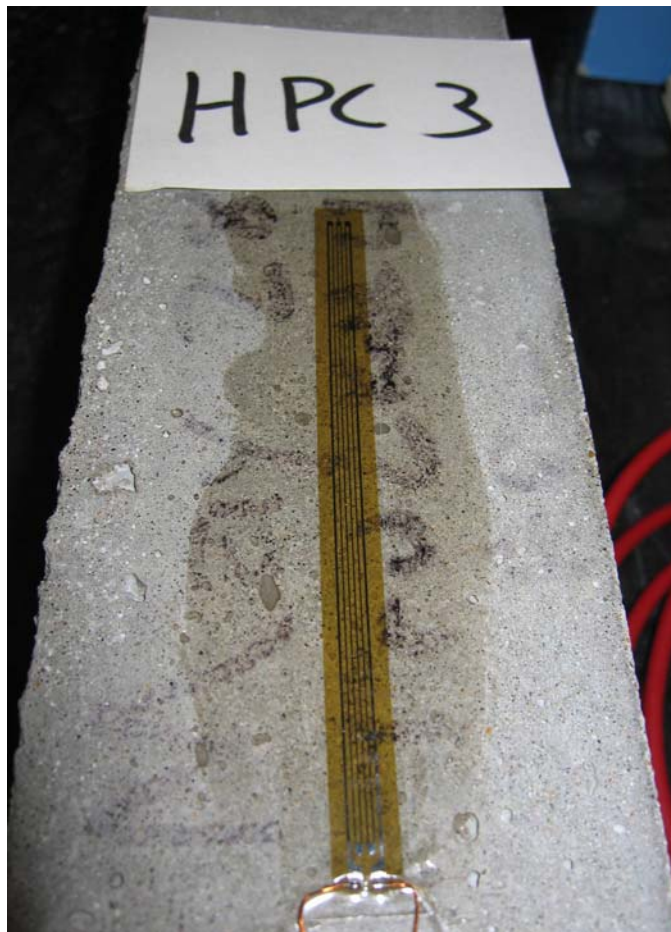
Figure 6. Typical Concrete Strain Gage Installation
