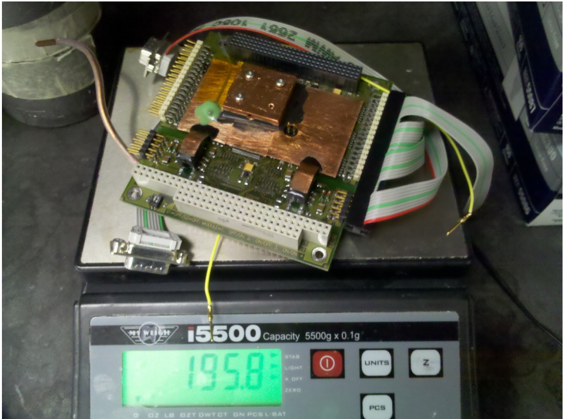
Figure 16: Flight Modified PC/104+ Board
