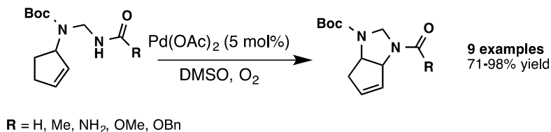
Scheme 2.5: \text{Pd}(\text{OAc})_2/\text{DMSO} Catalyzed Oxidative Cyclization of Amins
