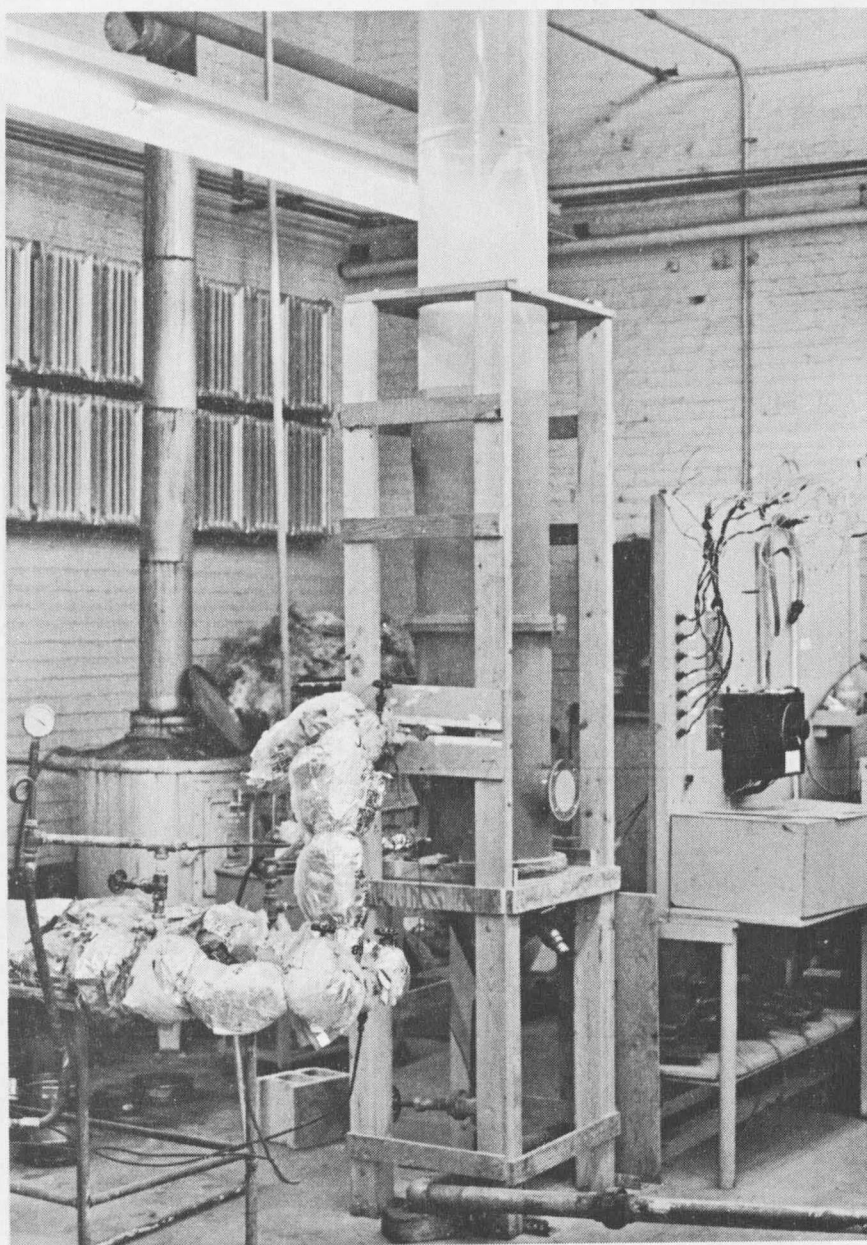
Figure 11. COLUMN OF COILED SPIRAL TUBE SYSTEM
