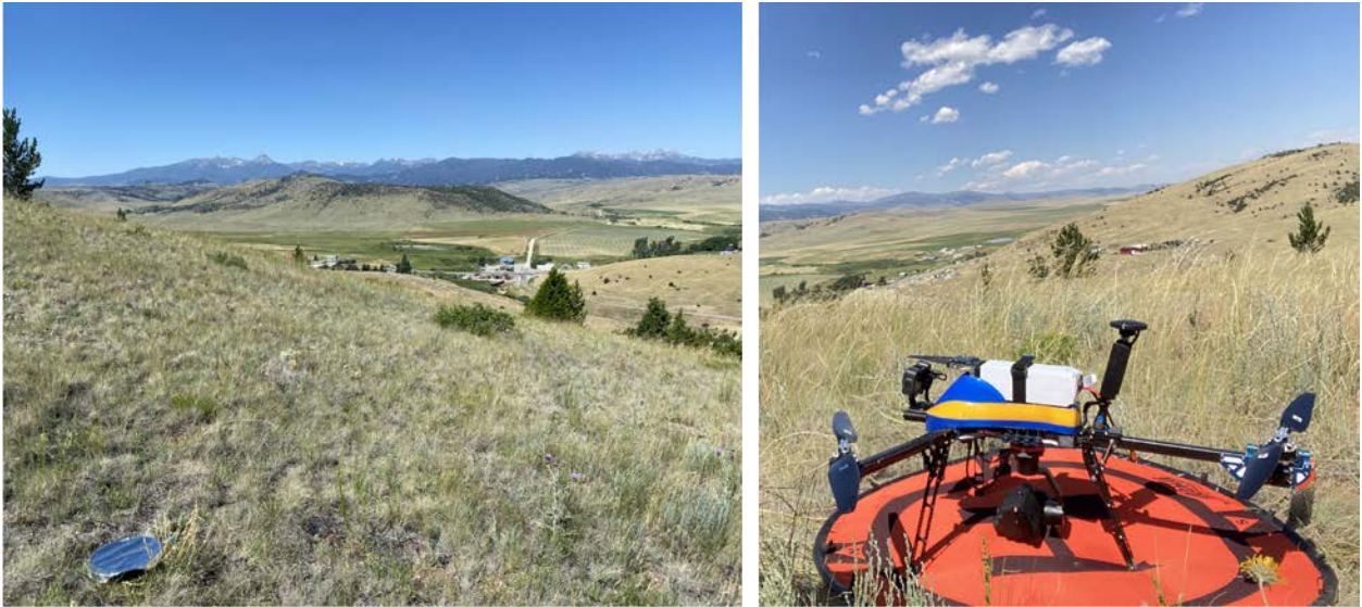
Figure 2.6: Left: GCP covered in aluminum foil, overlying one of the sampling locations. Right: The VisionAerial SwitchBlade-Elite tricopter UAV with the FDPR mounted on the gimbal.
