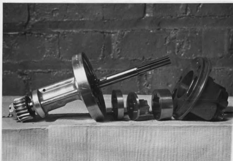
Fig.37- Lubricating Oil Pump
