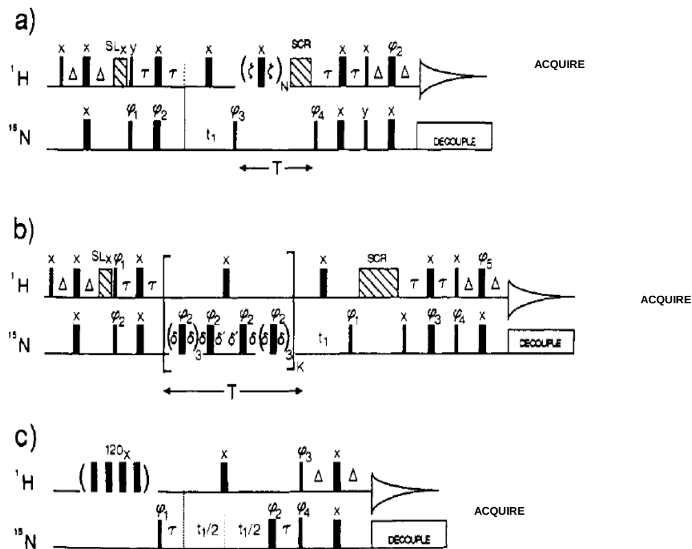
Figure 5. Pulse Sequences Used For The Measurement Of ^{15}\text{N} (a) T_1 and (b) T_2 Relaxation Times, And (c) For Measurement Of The ^{15}\text{N}\{^1\text{H}\} nOe In Our Studies. (47) These pulse sequences can be thought of (and read) as a schematic plot in time (increasing horizontally, rightwards) to perform each run of the relaxation experiments. The narrow and wide bars indicate pulses applied at 90^\circ and 180^\circ respectively. Phase cycling was used to suppress spectral artifacts in the data. This was accomplished by acquiring data with different pulse and receiver phases. \phi represents the phase of applied excitation pulse and x or y indicates the position of the receiver. \phi undergoes variations (cycling) throughout the pulse sequence. The order of variation is set to result in the minimization of artifacts after summation of the data from all of the scans in the cycle. Gradient pulses were also included in the pulse schemes to obtain coherence transfer selection but are not visible in the plots shown here. Pulses shown in striped boxes and labeled as SL and SCR represent high power pulses (short, \sim 2 ms and long, \sim 12 ms, respectively) refer to spin-lock and scrambling pulses respectively and are included to obtain higher coherence selection by dephasing of \text{H}_2\text{O} magnetization. To increment the relaxation delay, T , the loop counters N (for scheme a) and K (for scheme b) are incremented. In sequences a) and b), the T period is where the variable delay is implemented (inversion recovery). The composite pulse in duration T gets rid of the cross-correlation between dipolar coupling and chemical shift anisotropy by periodic application of 180^\circ ^1\text{H} pulses during the T_1 or T_2 relaxation period of duration T . In sequence c), the 120^\circ high-power pulses are applied during the entire delay between scans (3 s) at 20-ms intervals, to maintain a saturated state of the ^1\text{H} reservoir. For obtaining the reference spectrum without nOe, the 120^\circ pulses were omitted and, instead, two scrambling pulses of \sim 10 ms each, spaced by 1 ms, are introduced immediately prior to the 90^\circ ^{15}\text{N} pulse in order to eliminate the \text{H}_2\text{O} signal.
