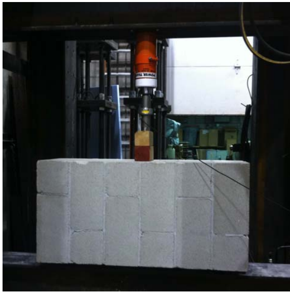
Figure 19. Tensile specimen prior to testing
