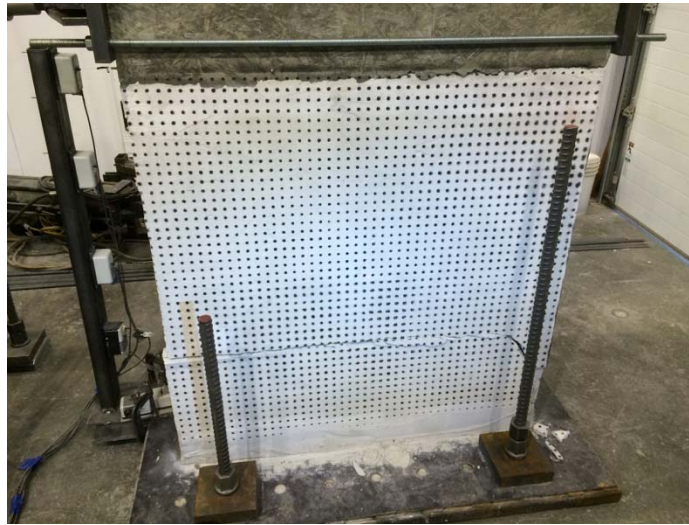
Figure 39. TS wall after failure
