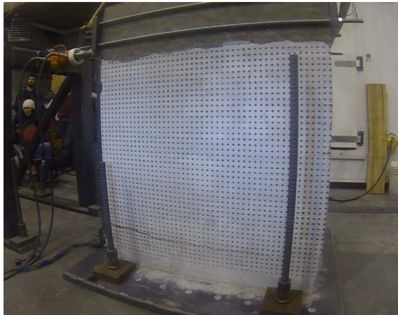
Figure 36. Failure surface of TPS wall
