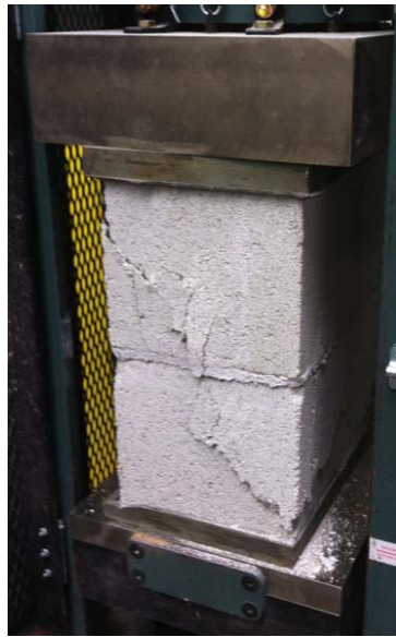
Figure 13. Typical prism failure
