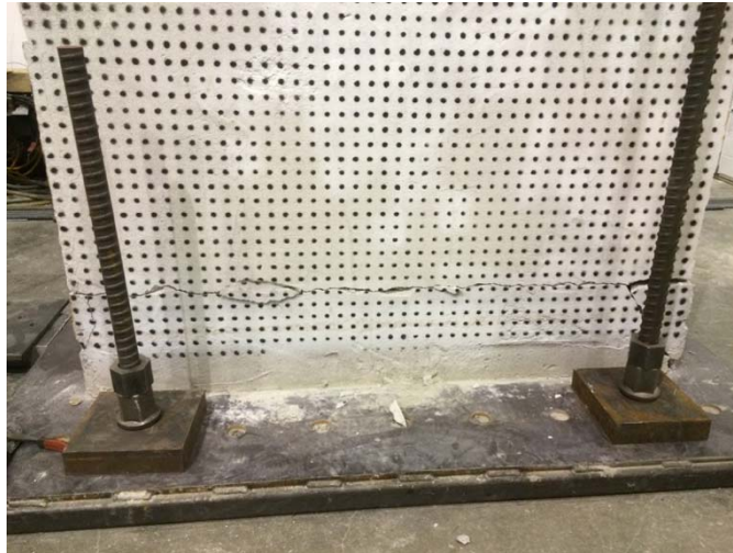
Figure 33. TP wall after failure
