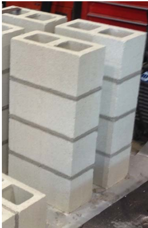
Figure 17. 4-block prism prior to grouting
