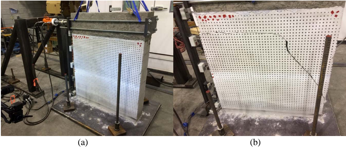
Figure 27. SP wall: (a) before loading and (b) after loading
