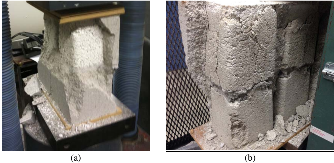
Figure 14. Ultimate failure of (a) perlite prism and (b) structural prism
