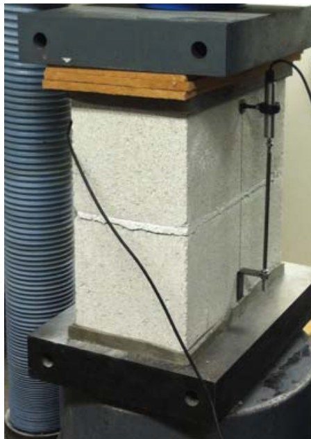
Figure 15. Modulus of elasticity test setup
