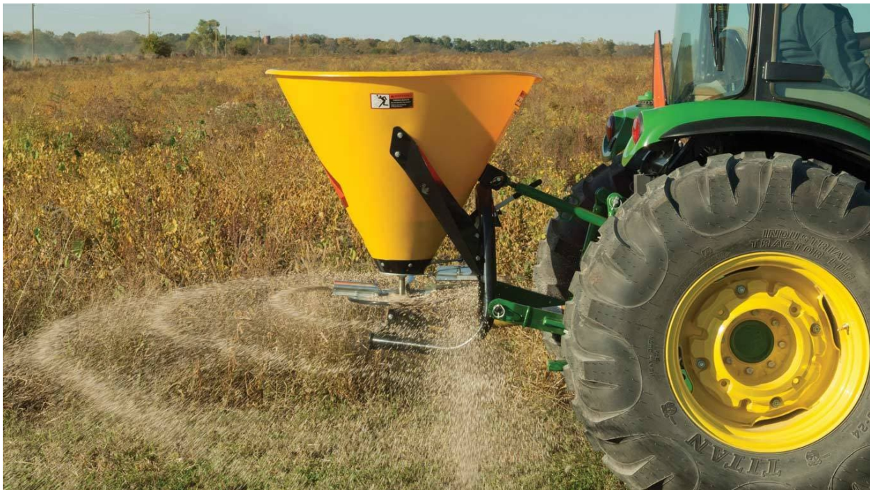
Figure 6. Broadcast seeder used in over-the-snow seeding. The seed is evenly distributed by the spinning disk on the bottom of the equipment. This seeding technique is used to inter-seed, and on sites that have extensive woody vegetation and debris. (photo from johndeere.com)
