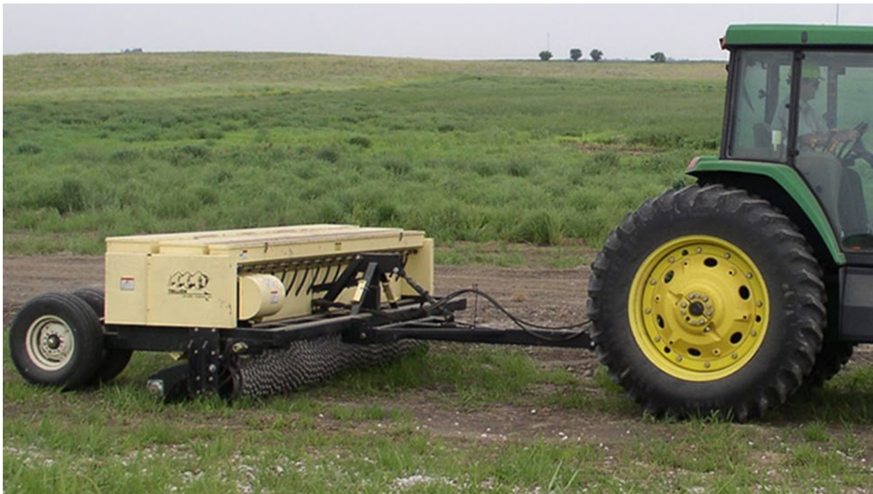
Figure 5. Tractor pulling the native seed planter (Truax Drop Seeder). This equipment is designed specifically to plant "fluffy" native seed. A conventional seeder would not work with prairie seeds. (photo from Truax.com)
