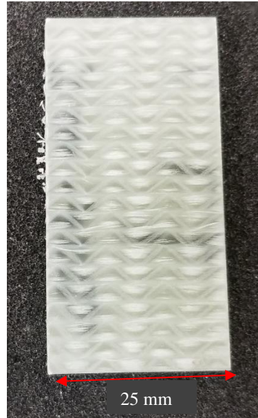
Figure 51. Glass fiber reinforced epoxy composite surface after sanding with FEPA 1000 grit sandpaper and etched with hydrofluoric acid (HF). The HF was applied to highlight the fibers for visual observation.
