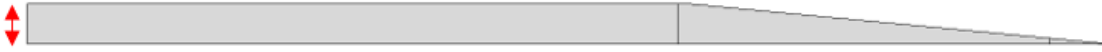
Figure 95. Left side of the scarf tension specimen with two partitions. The red arrow indicates the part thickness of 6.16 mm.
