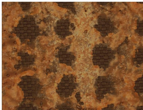
Figure 29. Failure surface of a DCB specimen contaminated with mold release [76].
