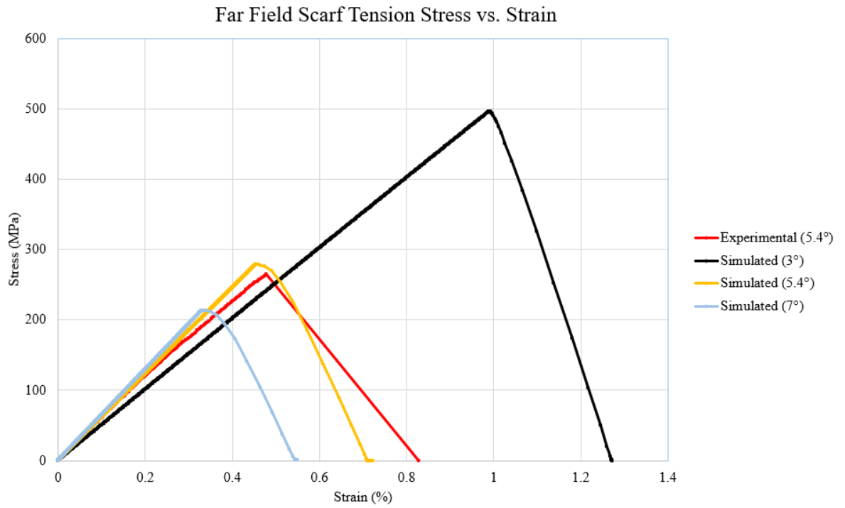
Figure 105. Scarf tension far field stress-strain curves comparing experimental and simulated results.
