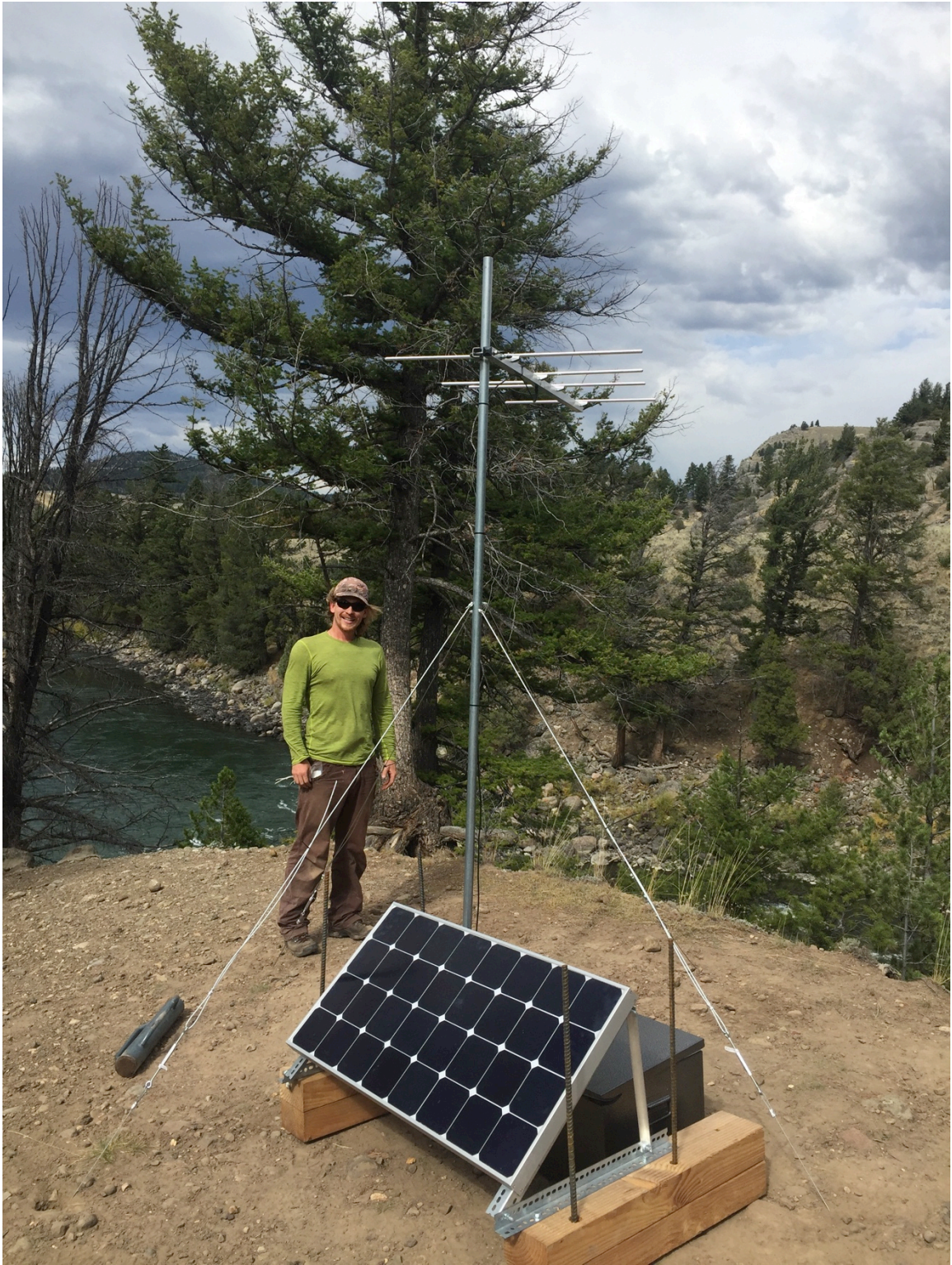
Figure 5.2. Fixed radio telemetry receiver station set up at the confluence of the Yellowstone River and the Lamar River.
