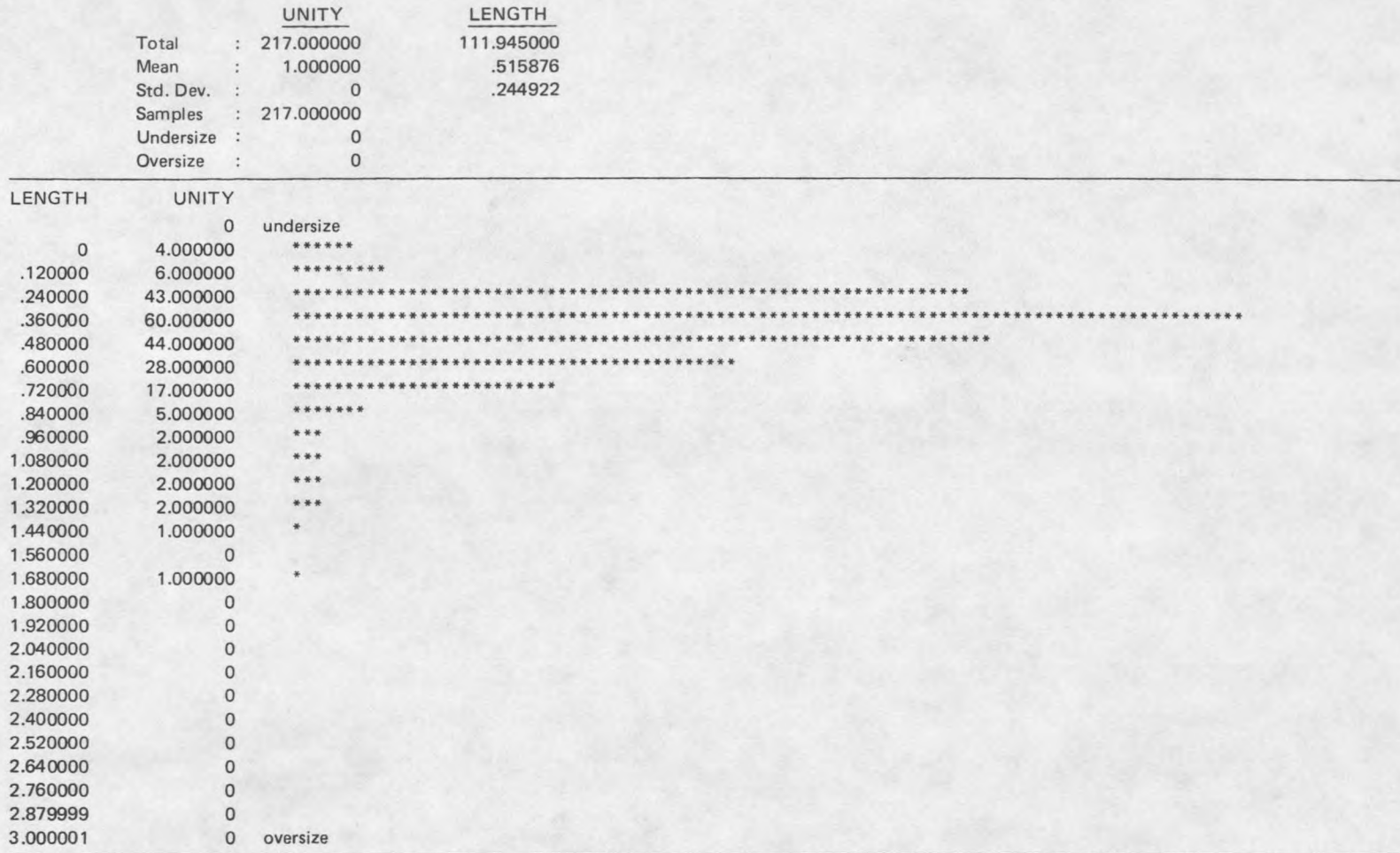
Figure 20. Linear distribution of unity by length, units of length in millimeters.
