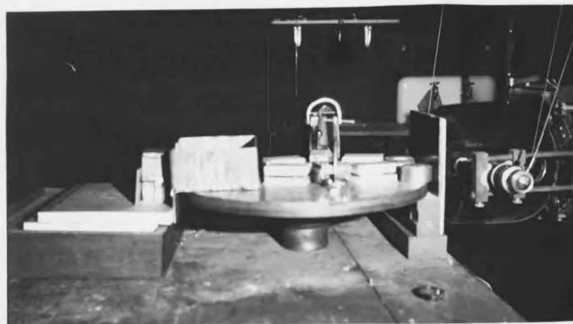
Figure 2b. SIDE VIEW OF APPARATUS. Shielding removed from one crystal.
