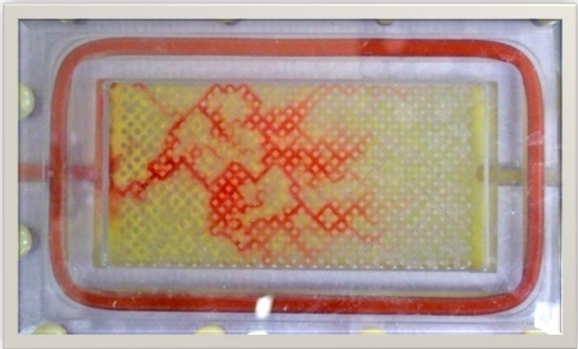
Figure 5.4. Pseudo steady state biofilm showing decreasing biofilm thickness along flow path
