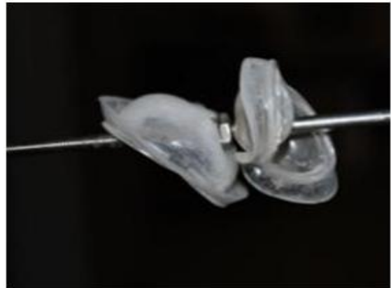
Figure B.4.2. Image of removed petri dishes that have been deformed by exposure to scCO_2
