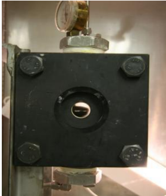
Figure B.4.3. Image of high pressure vessel, showing suspended aluminum trays inside.
