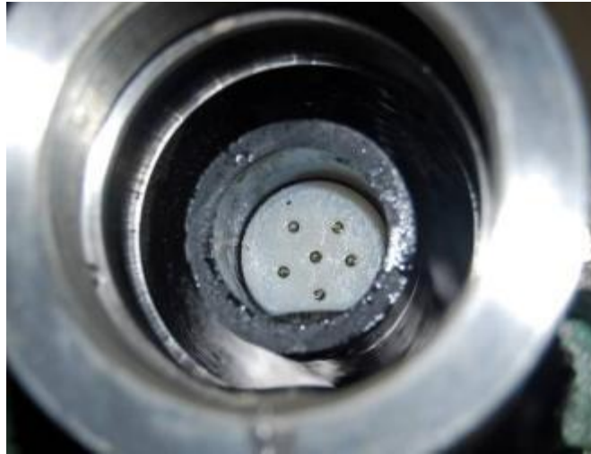
Figure A.2. Image of Hassler-type core holder. The black sleeve, which contains the white core inside, has an overburden pressure of mineral oil that was compressed with a hydraulic jack pump. The white core contains six glass tubes (1mm i.d.) simulating pores.
