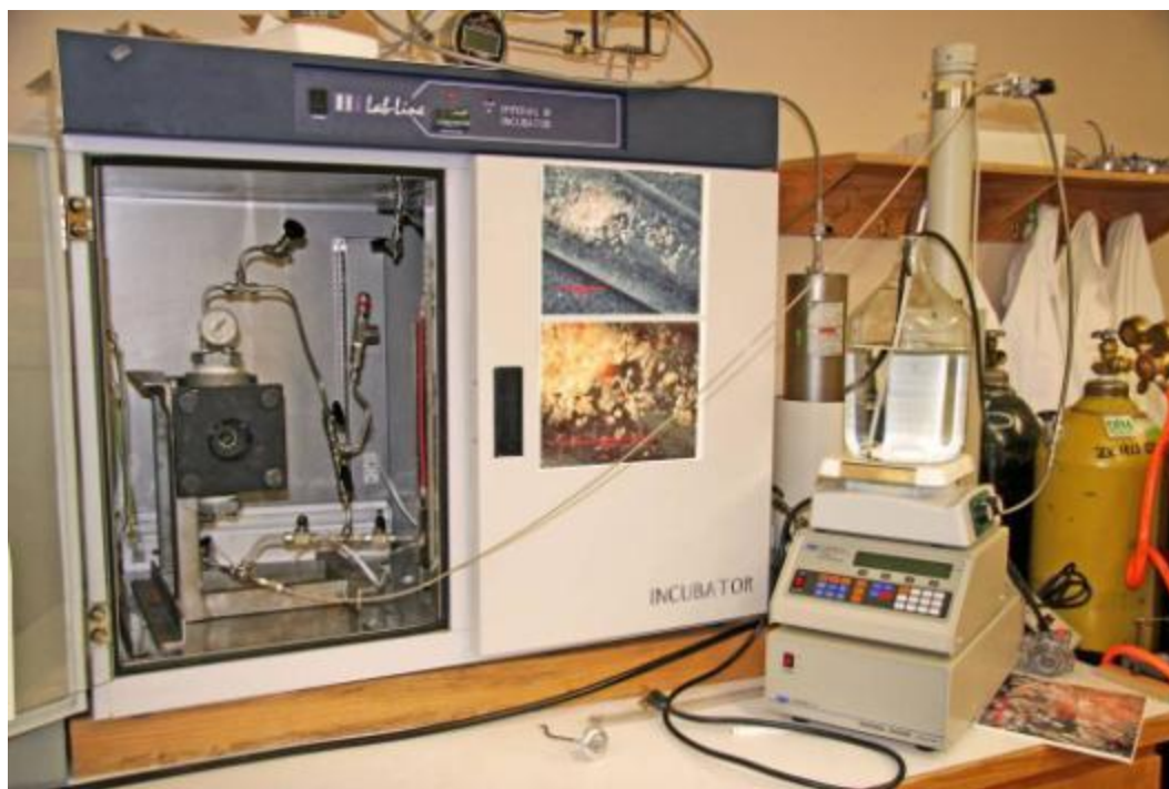
Figure B.1.1. Image of high pressure vessel system contained in an incubator. A piston accumulator is behind the right door.
