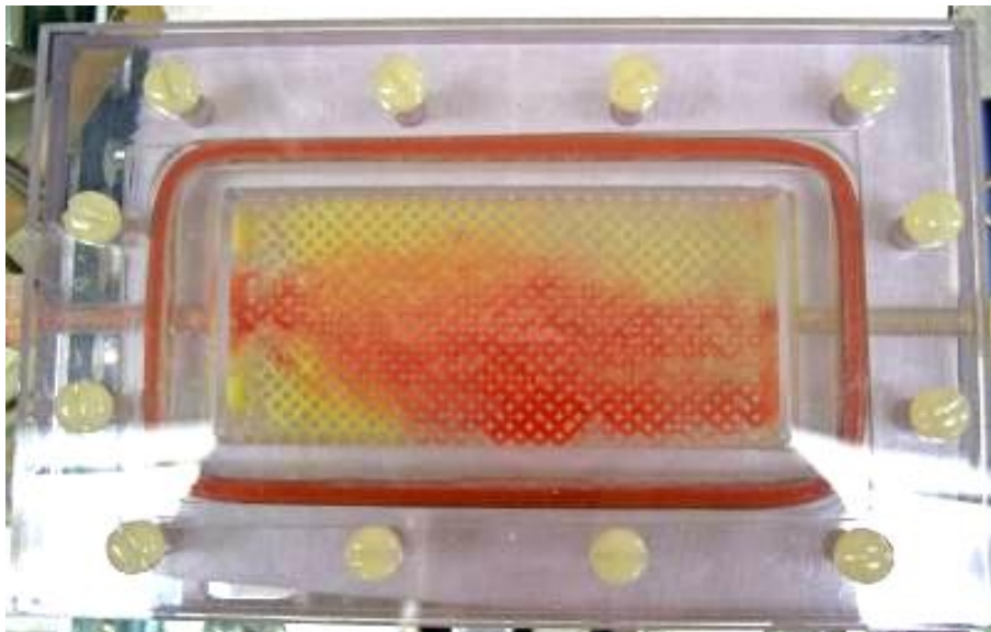
Figure 4.24. Constant flow reactor immediately following stagnant bleach exposure
