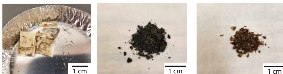
Figure D.9: Composted PLA samples after 20 days (left), PLA with 20% FW900 after 40 days (center) and neat PLA after 40 days (right).
