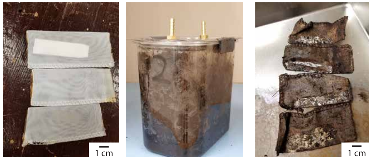
Figure D.2: Photographs of the setup for PLA and FW900 biochar composting experiments. (left) Samples in mesh bags prior to composting. (center) 2L polycarbonate container with compost. (right) Samples in mesh bags after 20 days of composting.
