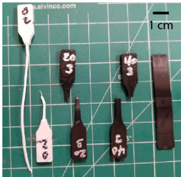
Figure F.1: Photographs of tensile samples with: (from left to right) 0%, 20%, and 40% biochar addition after testing and a flexural sample with 20% biochar addition.
