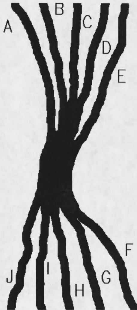
Figure 4. A cliff line formed by intersecting contour lines.
