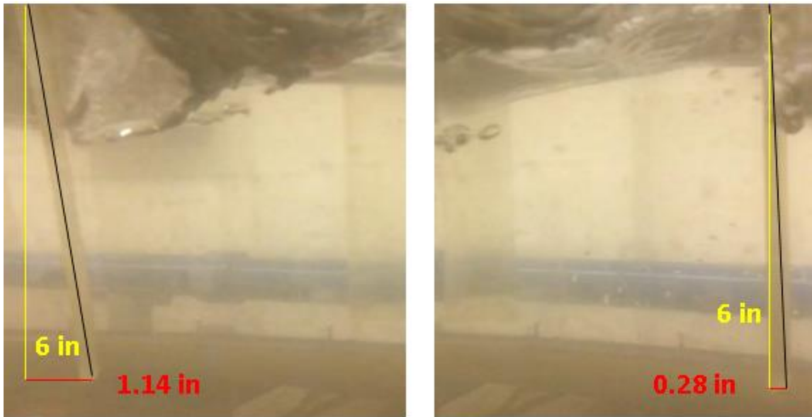
Figure 49: Experimental blade deflection: a) blade at 90^\circ , b) blade at 270^\circ
