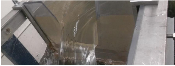
Figure 47: Full weir output with small metal weir clamped to flume
