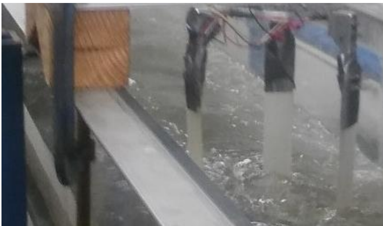
Figure 48: Turbine rig in flume test position
