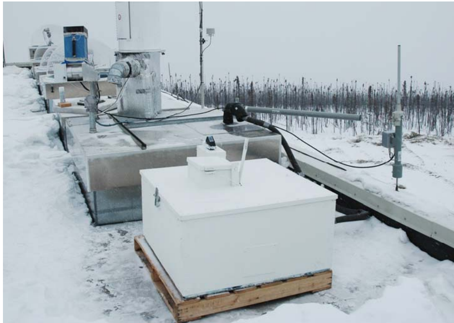
Figure 1-1. The original ICI during a deployment at Poker Flat Research Range, AK. The ICI camera and calibration equipment are inside the white housing in the foreground. The instruments in the background are other instruments at the site operated by other groups. (Photo by J. Shaw)
