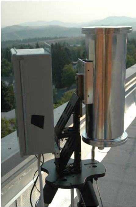
Figure 4-10. Prototype of the 50° fov second-generation ICI during the 2007 deployment at Bozeman, MT. The camera is inside the enclosure on the right and the electronics are in the box on the left. In the photo the front plate with the IR window is on the enclosure. (Photo by J. Shaw)
