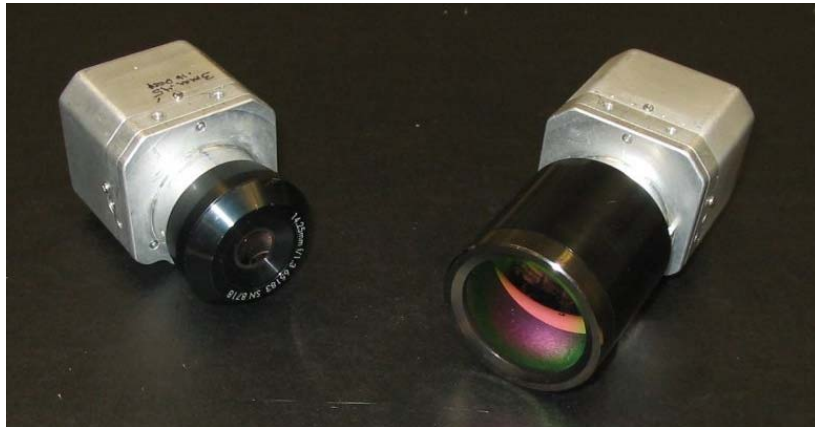
Figure 2-8. The Photon Core thermal cameras built by Indigo Systems: (left) the 50° fov camera, and (right) the 100° fov camera.
