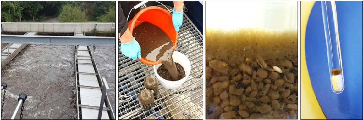
Figure 9.2. (Left to right) Samples were collected from the Utrecht wastewater treatment plant's Nereda™ sequencing batch reactor. The granules settle first with the floccular sludge on top. A single granule was then placed in a 5 mm NMR sample tube for imaging experiments.
