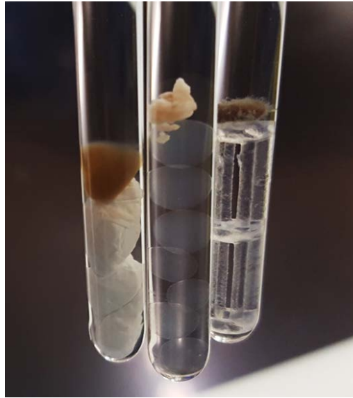
Figure 9.3. The granule samples were placed in 5 mm NMR sample tubes, elevated with either Teflon tape (left), a stack of alginate beads (center), or a 3-D printed frame (right). The granules shown include an extracted EPS granule, a VFA-producing laboratory grown granule, and an anammox granule from the B-stage of Dokhaven treatment plant.
