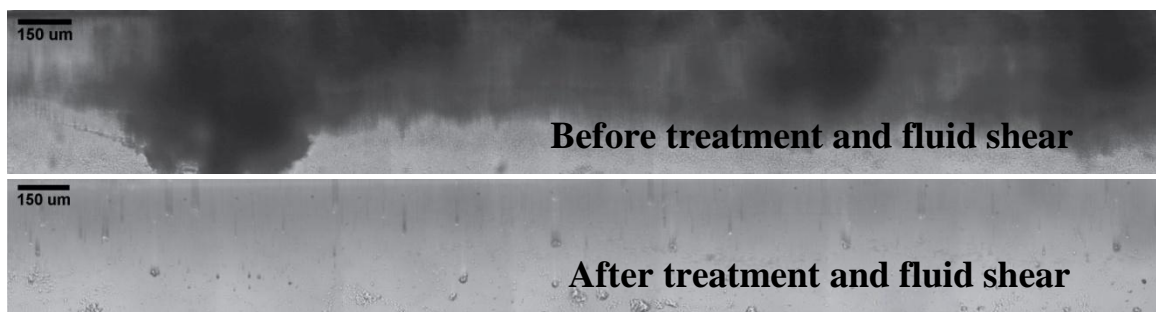
Figure 50) S. epidermidis biofilm pictured along the length of the capillary flow cell reactor before and after induced with fluid shear and 0.1 molar urea treatment
