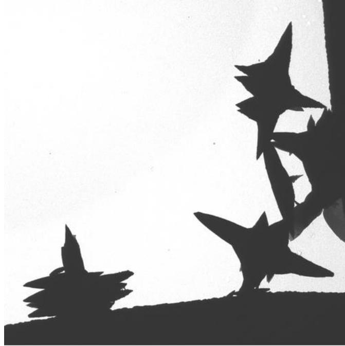
Figure 5.19 TEM image of agglomerated Sigma Aldrich nanoparticles prepared at neutral pH. The sizes of each were not recorded, however the structures are on the 10-100 \mu\text{m} scale. The extended structures along the bottom and right are the copper wire grid used to hold the TEM samples.
