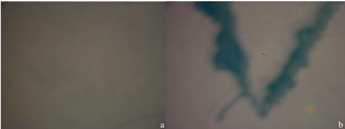
Figure 3.11. Images showing an ideal PMMA layer spun onto a sample. Hardly any deformities were seen on the LN after the sample had been cleaned with solvents and re-spun.
