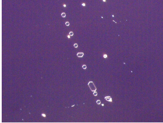
Figure 5.5. Poled pattern found on a sample that had been patterned with a chromium mask, but not intentionally poled through AOP.
