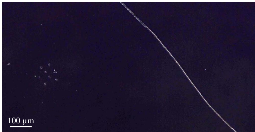
Figure 5.6. Image of poled cluster near scratch in lithium niobate sample.
