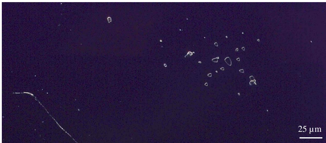
Figure 5.7. Image of poled cluster near scratch in lithium niobate surface.
