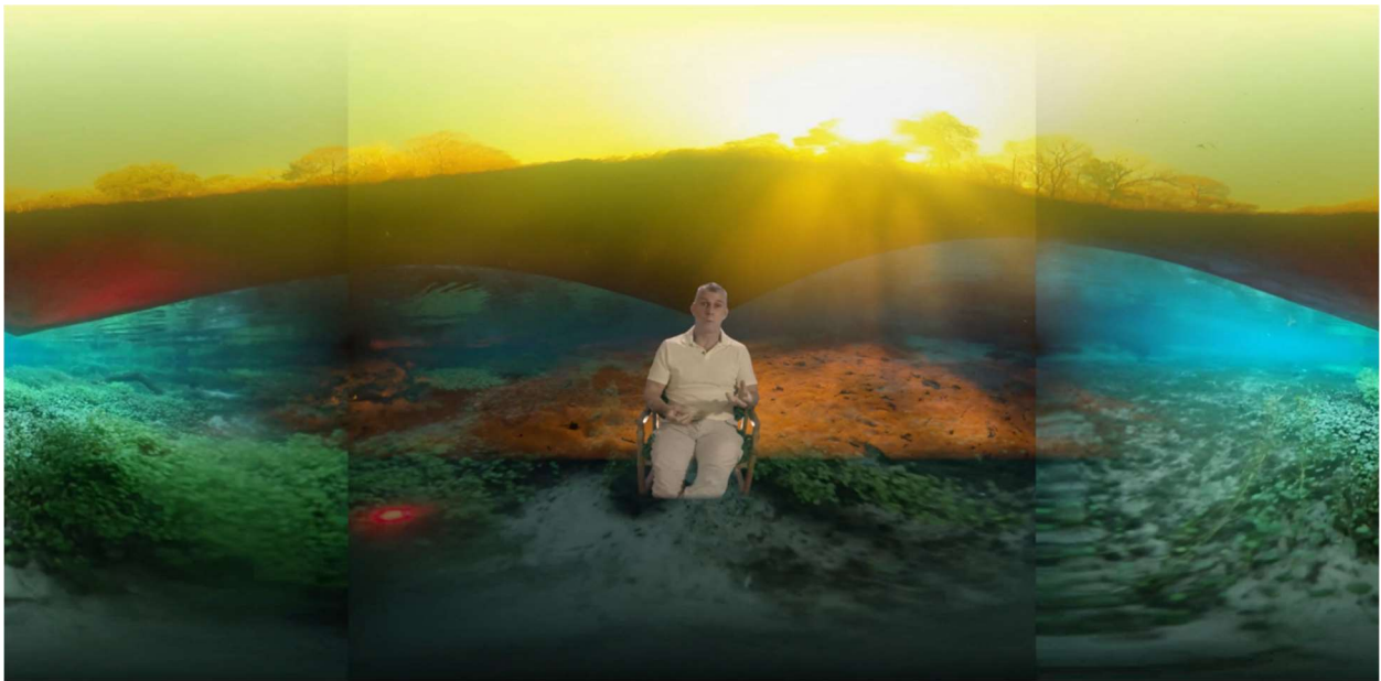
Figure 2: The two vertical lines dividing this frame form one circular seam when projected to a sphere for playback. The seam is the result of a blind spot of about 10^\circ on the camera rig.
