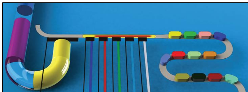
Figure 1.6 Assembly line formation of drops with spatial barcoding. A valve system allows a fraction of an incoming sample plug to enter while reagents are injected [38].
