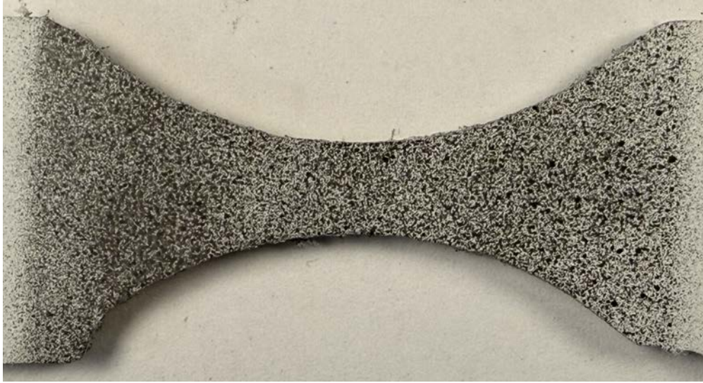
Figure 10: Fiberglass double notch sample painted with the ideal black and white finish for DIC testing purposes.
