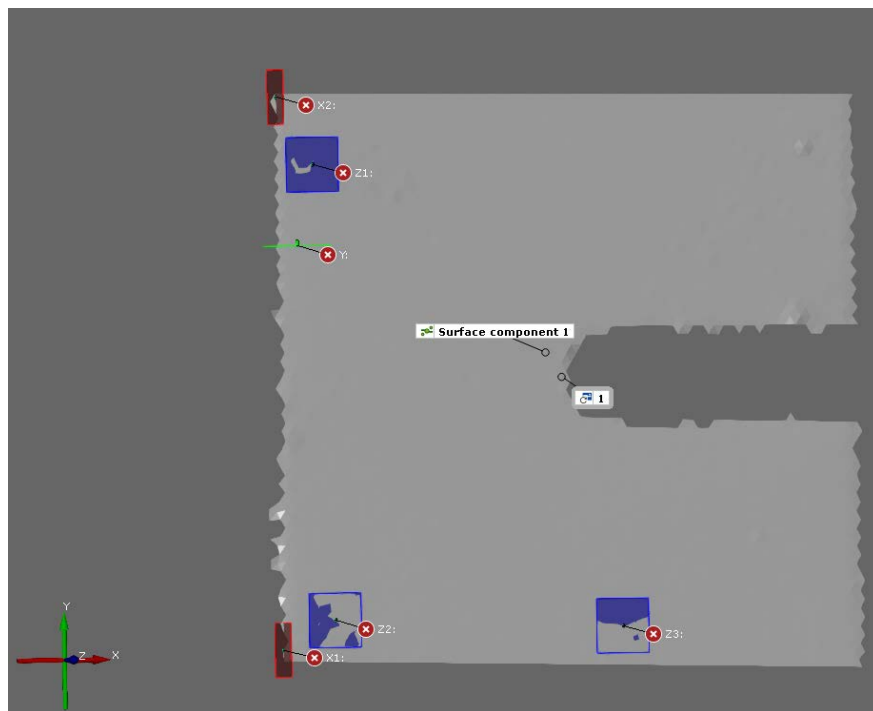
Figure 14: Coordinate plane defined on the surface component of a coupon in Aramis.
