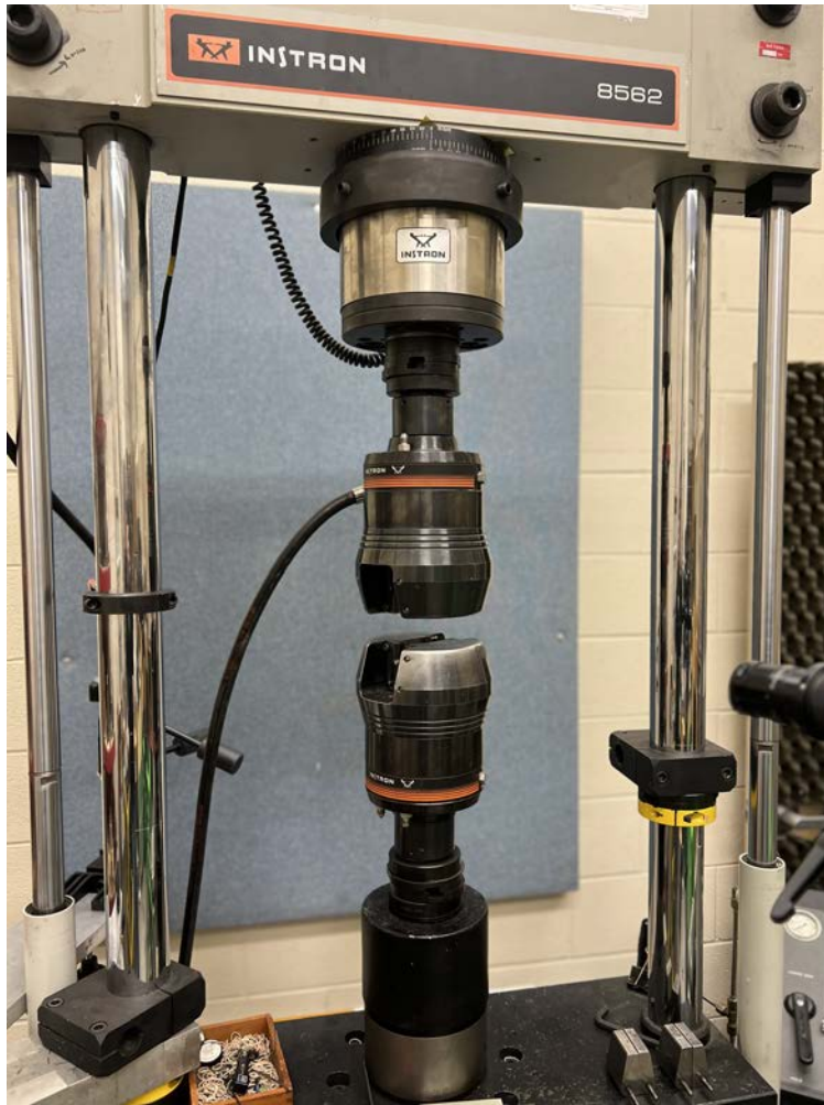
Figure 8: Instron 8562 system used to displace coupons in exclusively the y direction if the IPL could not invoke failure within the same test.
