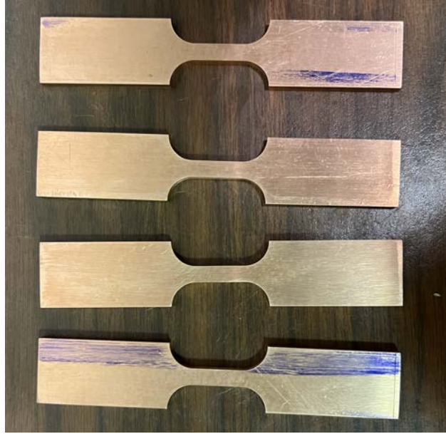
Figure 9: Example copper 110 coupons machined to be tested in tension for testing verification.
