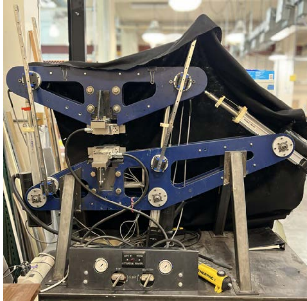
Figure 4: The IPL used to pull coupons multiaxially based on instructed displacement inputs of x , y , and z directions.
