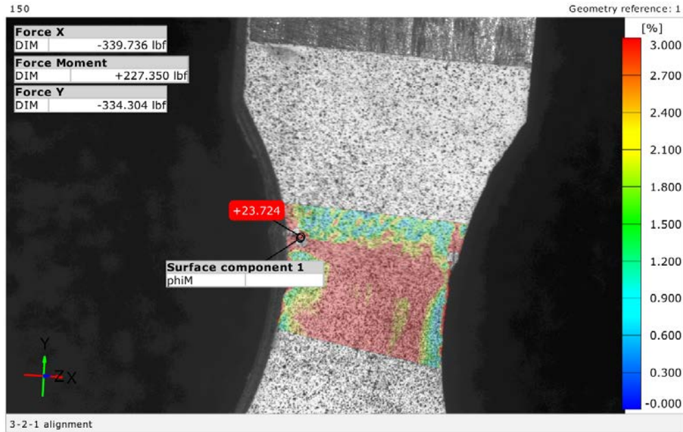
Figure 22: Uniaxial T8 failure pattern as seen through the \phi_M strain concentrations in Aramis.
